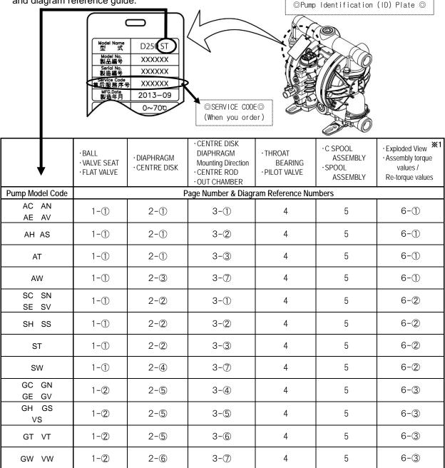
× 1)Before operating the pump for the first time please re-torque all bolts. Also re-torque bolts if leaks are discovered as part of the daily inspection regime.
